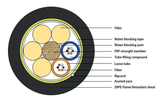
AR-1-FADPE-ZR-ADSS-100/200M-xxF G652D Structure of other fiber counts refer to 3.4 Schematic for reference only
