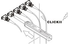
Be careful not to slant the One-Click Cleaner SC while inserting into the adapter.
