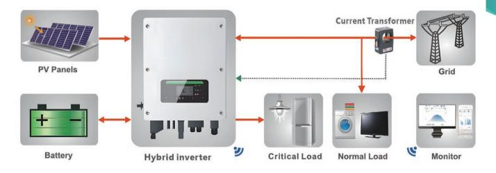
On and off grid solar system includes solar panels, on and off grid hybrid solar inverter, lithium ion batteries. It not only can supply electricity to user 's home appliances, but also can set the ex cessive electricity to be charged into the batteries or sent to the mains grid.
